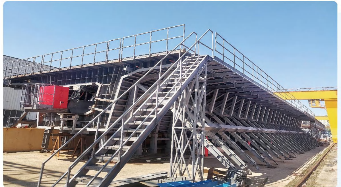
韩国高铁 40 米箱梁模板 BOX GIRDER FORMWORK (40 M) FOR A HSR PROJECT IN GWANGJU, KOREA
