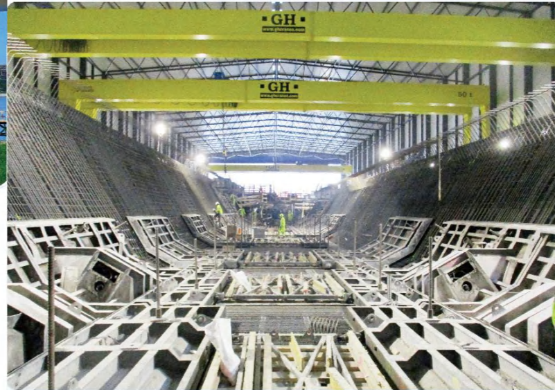
丹麦 73 米桥梁箱梁模板 BOX GIRDER FORMWORK (73M) FOR A BRIDGE PROJECT IN DENMARK
